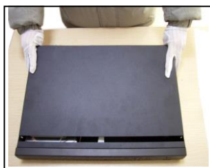
2. Disassemble the cover
