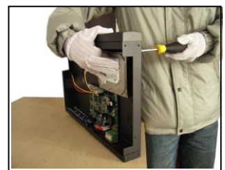
3. Fix the screw of hard disk
