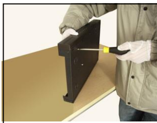
4. Fix the screw of hard disk
