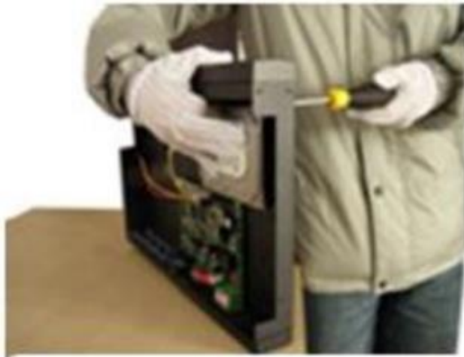
① Use Screws to fix the HDD in the board.
