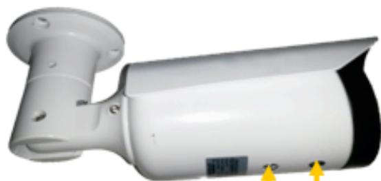
You can adjust the focus and the zoom by turning the two small screws that are directly attached to the lens. ✓
