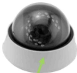
Simply anchor the bottom plate of the camera and gently twist the white plastic section counter-
